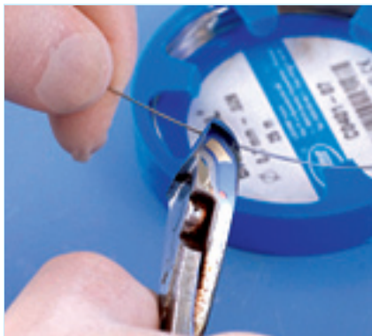
10CM OF 0.7MM STAINLESS STEEL WIRE
